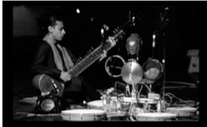
Figure 1. MahaDeviBot communicating in real-time with a performer using sensor on the ESitar and audio analysis.
